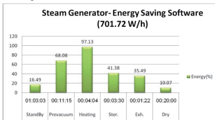
**In conclusion**, Celitron's Sterilizers reduce power consumption to the minimum. The use of a **Steam Generator** enables energy saving of ~20%. The **Energy Saving software** enables a drop of 12% more. Therefore, the Sterilizers are capable of reducing consumption by ~32%. When comparing to other Sterilizers on the market, Celitron's Sterilizers use 40% less energy.
