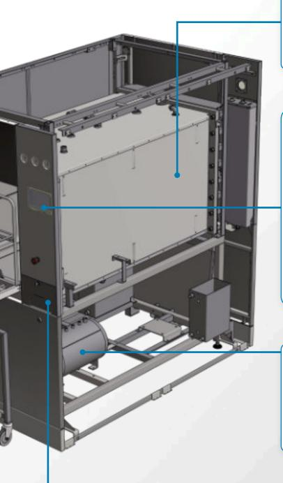
CHAMBER — The vessel is a double full jacketed square chamber, made of corrosion-resistant stainless steel 316L. It has large capacity from 110-880 Liters. Sterilization temperatures between: 121°C and 134°C
