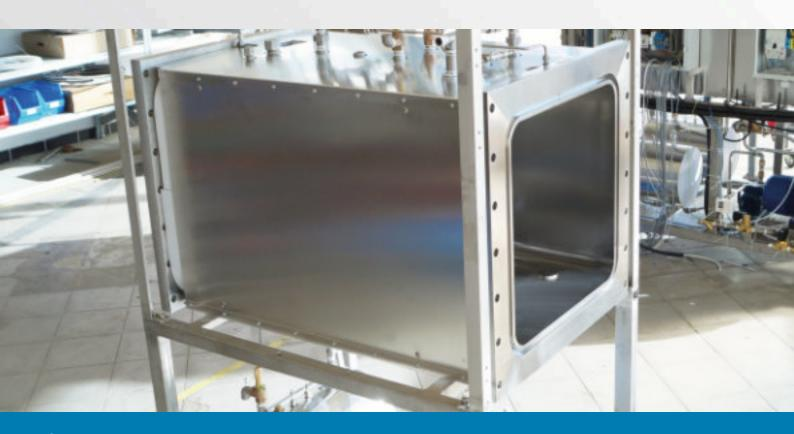
FU). The autoclave's framework and piping are also made of stainless steel. The highly efficient, high quality Hanno-Tech insulation material releases no particles; hence the Azteca A steam sterilizers can be used under clean room conditions. The advanced insulation technology further contributes to the high energy efficiency of the units.
